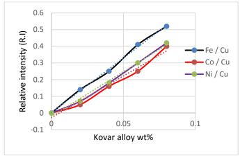
Figure 4: Calibration curves for Kovar alloys in organic liquid
