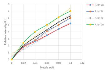
Figure 2: Calibration curves for pure metals in organic liquid
